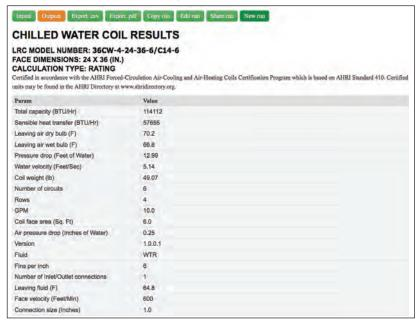
Use LRC's *On-Line Coil Capacity Calculator* to determine the capacity of your HVAC equipment instantly.
